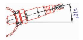
Recommended materials for the mating thread in the exhaust pipe \*: THexagon > 600°C or TGas > 930°C
